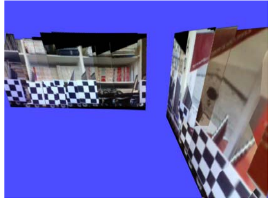
Fig. 9. Experimental results: OpenGL 3D view of the mapped environment. The chess board pattern could be cut off the map without loss of information postprocessing the obtained data or using stereo vision.
