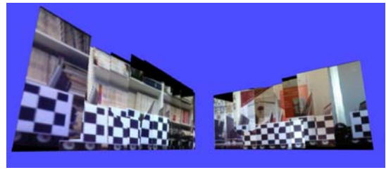
Fig. 11. Experimental results: perspective OpenGL 3D view of the mapped environment. The image coincides with a portion of the image that a camera would have taken if placed in the environment at the corresponding position.
