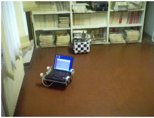
Fig. 7. Experimental set: MR follows the wall and brings the chess board pattern while OR localizes it and builds the map.
