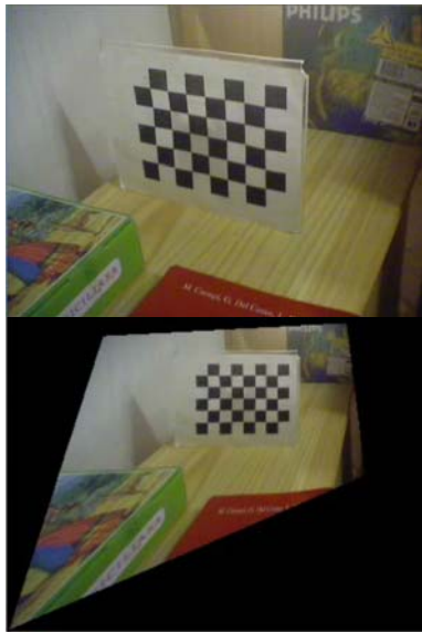
Fig. 4. Perspective projection inversion example: homography from image plane (top) to chess board plane (bottom). If all the elements of the top image would lie on the chess board plane, the bottom image coincides with a portion of the image that the camera would take when placed with focal axis perpendicular to the chess board. In fact, squares of the chess appear to be exactly squared.
